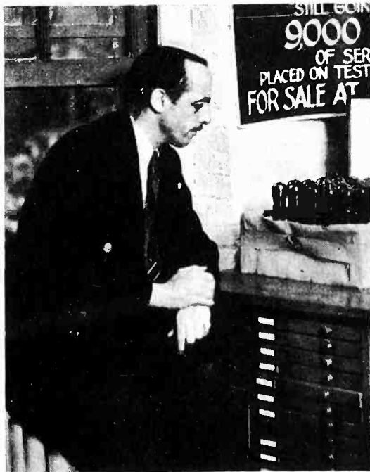
George Lewis, vice-president and chief engineer of Arcturus Radio Tube Company, Newark, N. J., examines 25 Type-127 detector tubes which have been on life test over a year—16,000 hours, more than 16 years of average service
